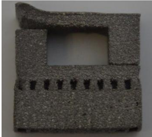
Figure 11. MANUFACTURED OVERHANG PART WITH CONTACT-FREE SUPPORT CASE 2
