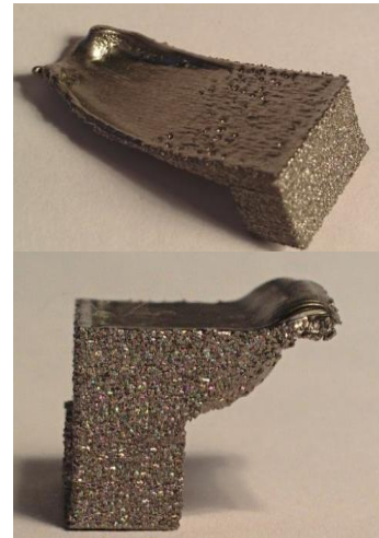
Figure 3. THE CURLING DEFECT
