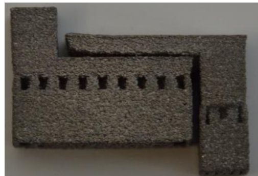
Figure 10. MANUFACTURED OVERHANG PART WITH CONTACT-FREE
